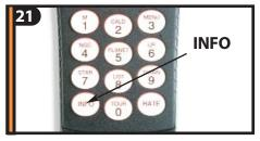
Press INFO to read information about the object displayed. Press the DOWN scroll key to display the next object. Press ENTER to slew (move) to the displayed object.
